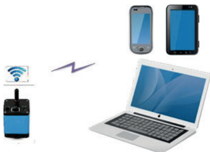
Figure 4 The PC or Mobile Device Connect to the Camera through WiFi AP Mode
