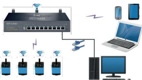
Figure 5 Multi cameras connecting to the router through the WiFi STA Mode
