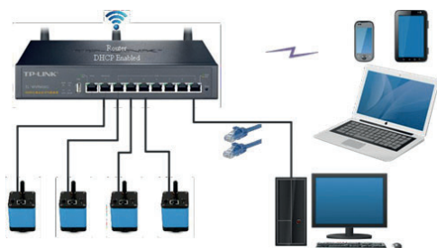
Figure 6 Multi cameras connecting to the router with the LAN method
