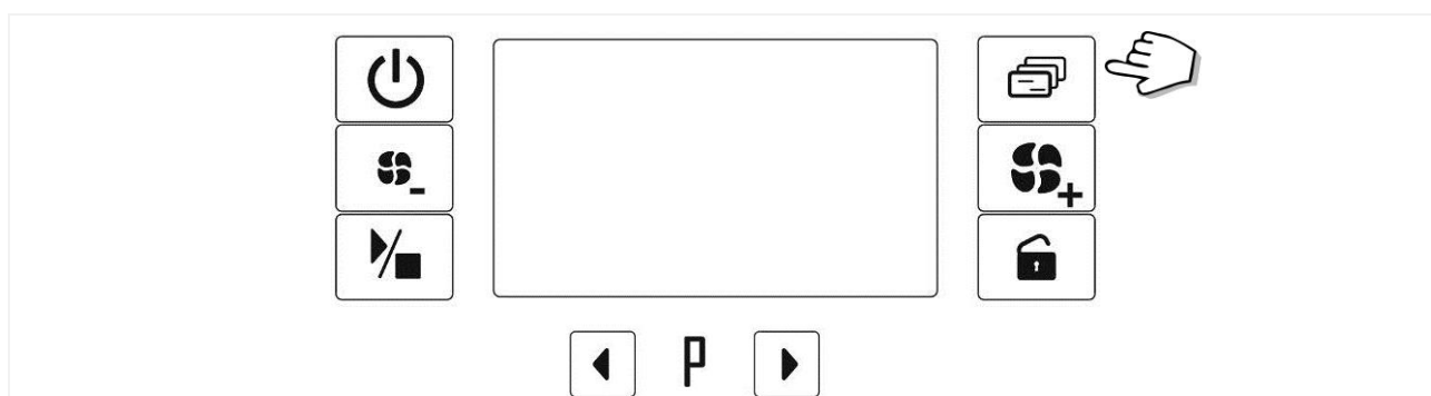
fig. 27 – Functions button: hold down to access the Setup mode.
