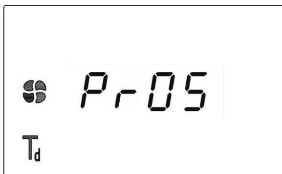
fig. 12 – Example of a Display screen . Program 5 selected The program includes a drying phase – Drying LED on . The program includes a thermal disinfection phase – "Td" LED on .
