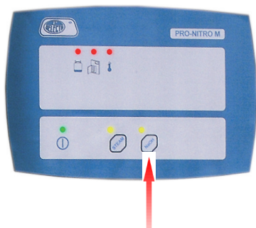
Manual NaOH adding during distillation
