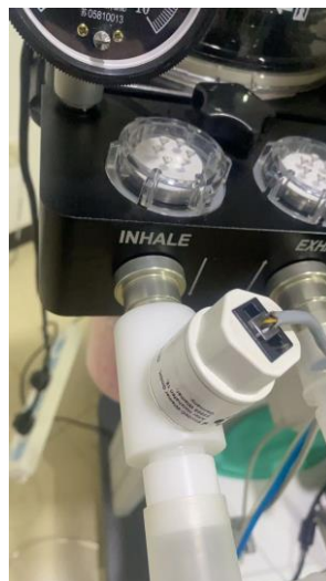
2-8 The another end is connected to the inhalation port of the anesthesia machine.
