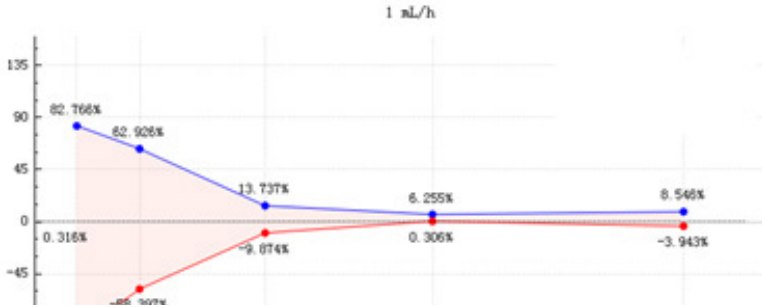
Graph 3 Trumpet curve: Percentage variation E_p against observation window duration P (min) and the overall mean percentage error A plotted from data gathered during the second hour of the test period
