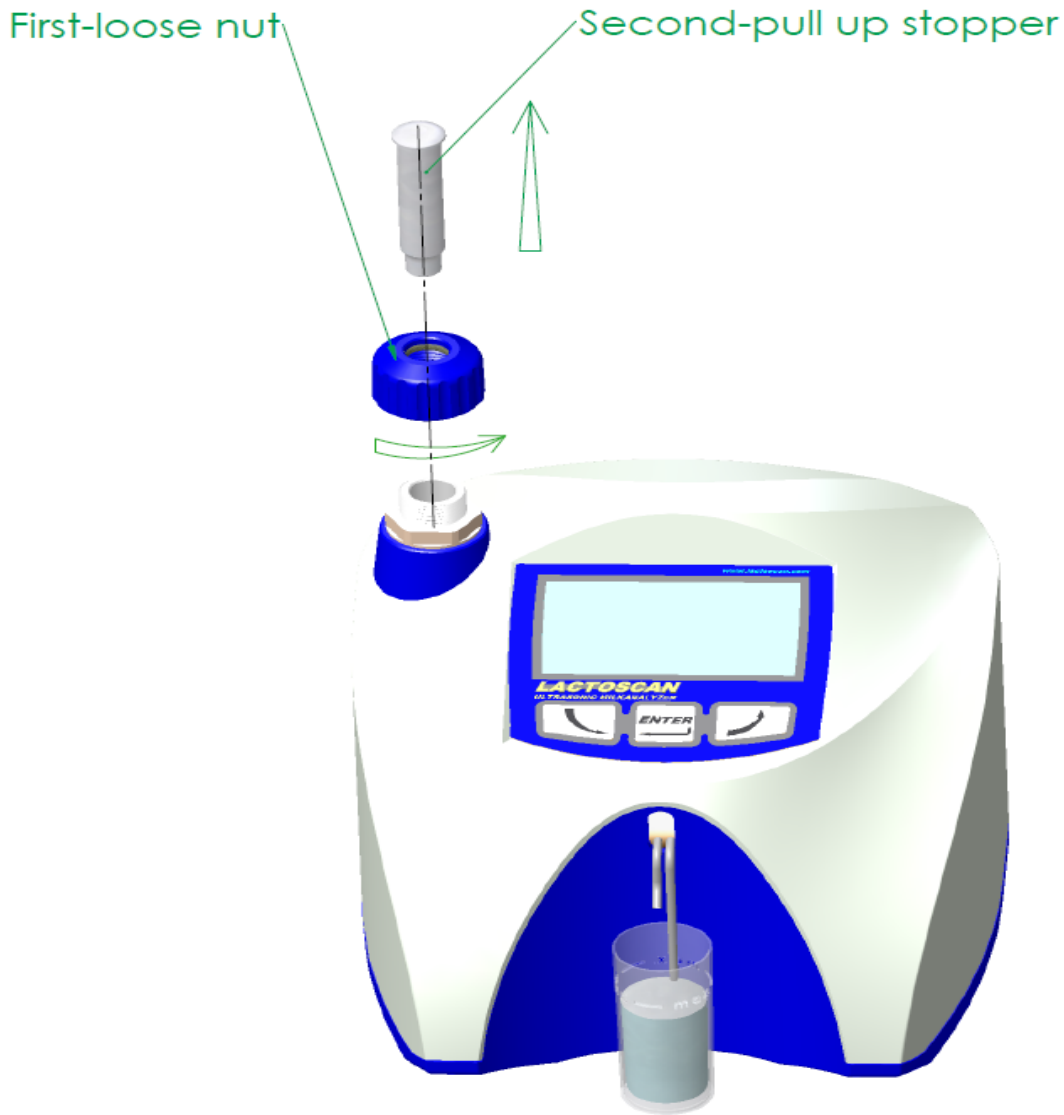
Fig. 7 Placing the stopper
