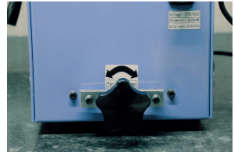
[Handwheel] Distance and stroke adjustment mechanism, allows the paddles to be moved forward and backward.
