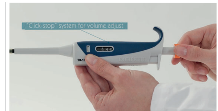
“Clik-stop” mechanism of volumen selection
