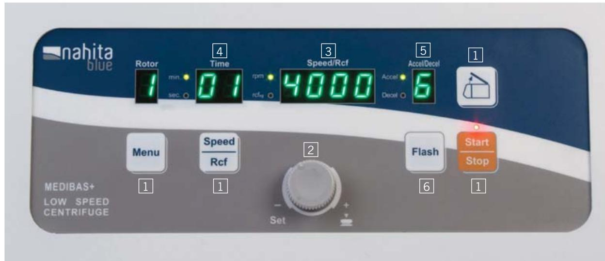
[1] Start/Stop, speed/RCF, parameter selection and lid opening buttons
