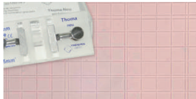
[2] WITH CLAWS: Similar to the standard format but with two claws that ensure optimal holding of the coverslip.
